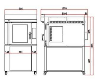
Model: BSM-5DHX Heating Way: Electric Power: 9KW Voltage: 105-110V / 220-240V / 380-415V N.W: 230KG Material: 1.2mm thick stainless steel shell, inner chamber 1.5mm thick 201 mirror panel stainless steel Capacity: 5 trays of 400\*600mm (15.75 x 23.6 inch) \* Other applicable baking tray sizes 460\*720mm Maximum (18 x 28.3 inch) 460\*660mm (18 x 26 inch)
