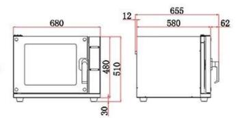
Model: BSM-4D Heating Way: Electric Power: 4.5KW Voltage: 220-240V N.W: 38KG Material: 1.2mm thick stainless steel shell, inner chamber
